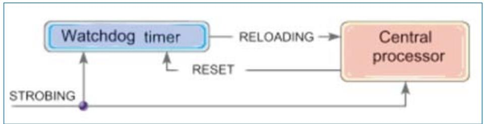
Fig. 4. A principle of the serviceability monitoring of the microprocessor with the help of the watchdog timer.
