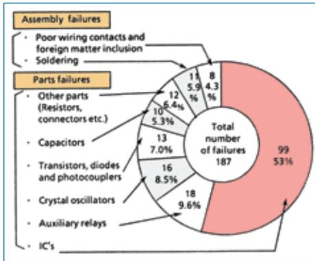
Fig. 2: The statistical data on damaged MPD based on investigations by leading Japanese companies [18].
