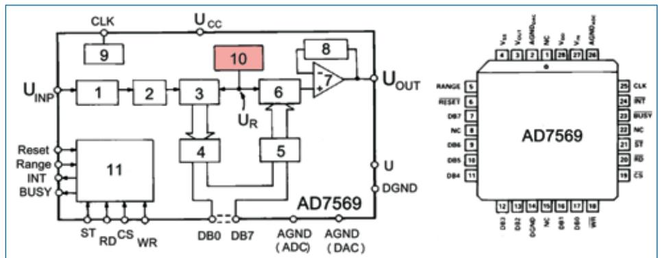
Fig. 3: Structure of the analogue digital converter AD7569 type. 1 - range network; 2 - unit of tracking/holding; 3 - analogue digital converter (ADC); 4 - ADC latch; 5 - DAC register; 6 - digital analogue converter (DAC); 7 - the amplifier; 8 - range network; 9 - synchronising clock; 10 - reference power supply.
