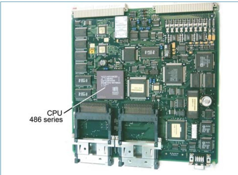
Fig. 7: CPU of the of central processor unit of the MPD series RE \*\_316, manufactured by ABB.
