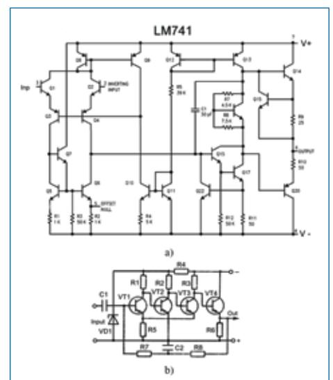
Fig. 1: Circuit diagrams of two amplifiers: at the top of a widely used IC LM741 type containing 20 transistors; below - the amplifier on the discrete elements with same parameters, containing only four transistors.
