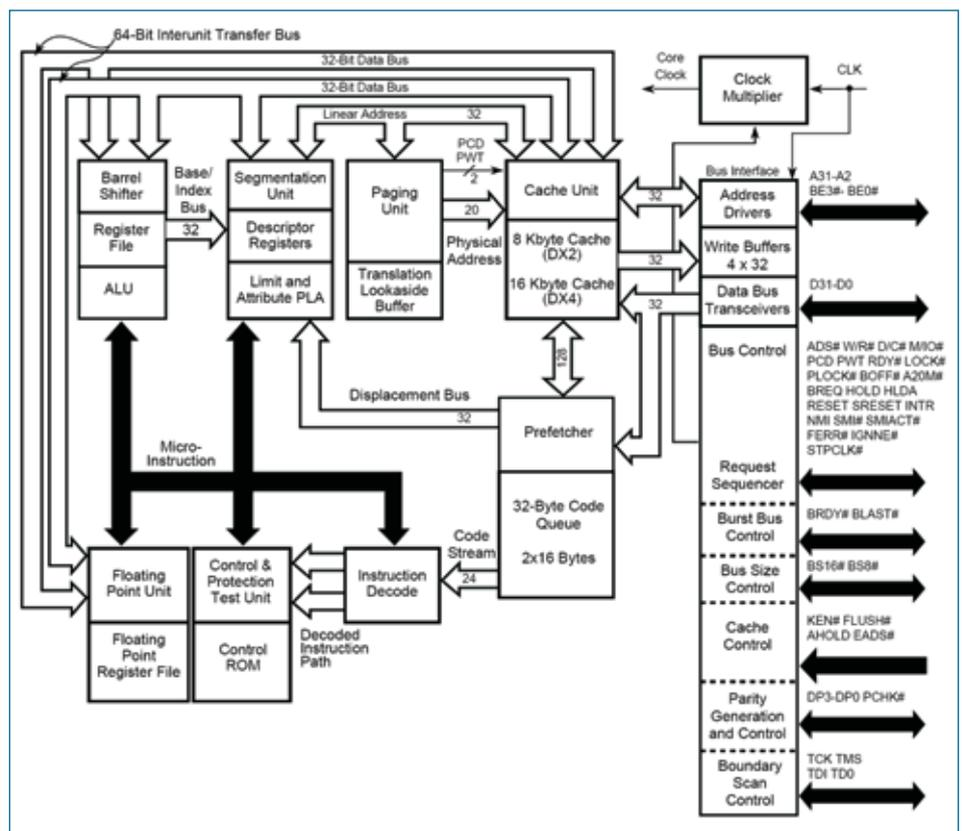
Fig. 5: Intel 486 SX block diagram.
