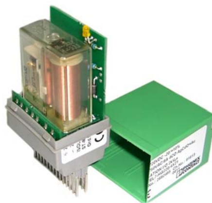
Fig. 15. ST-REL7-HG220/4X21 (Phoenix Contact) auxiliary relay type with the additional electronic components installed on the PCB inside of the relay case
