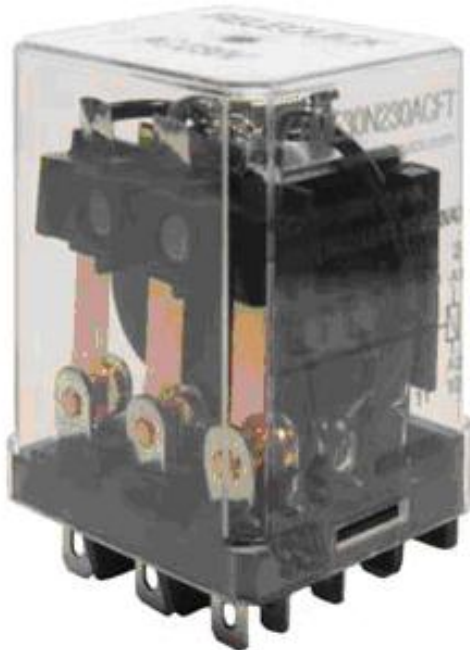
Fig. 10. The RMEA-FT-1 (RELEQUICK S. A.) relay type with one triple make contact, capable of switching currents up to 3A in an inductive load at 220VDC
