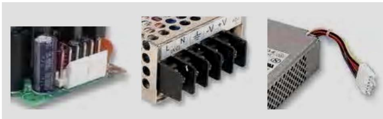
Fig. 11. Some types of the input/output connections used in SMPS
