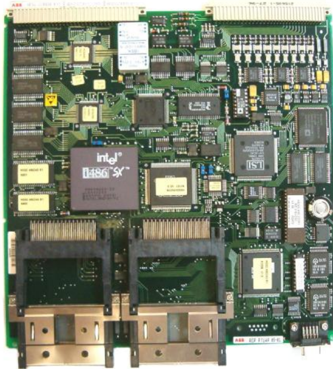
Fig. 1 - Main board of the MBR series RE_*316 based on computer chip Intel-486.
