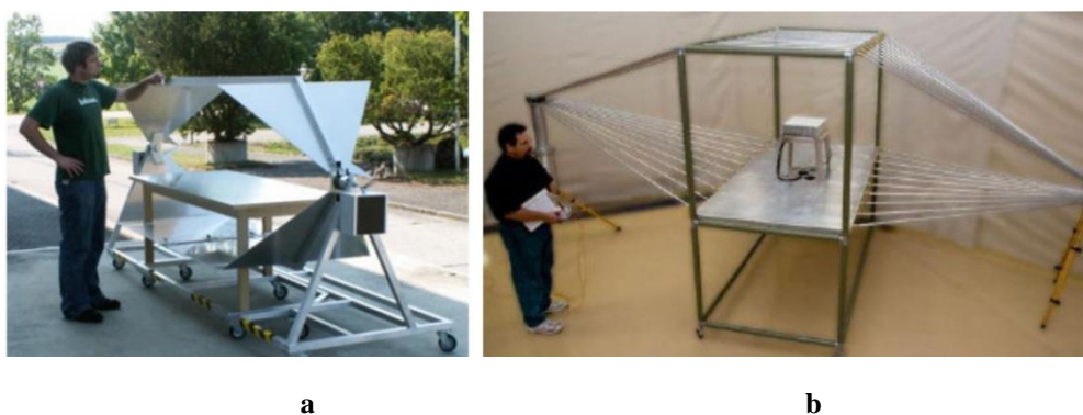
Fig. 10. Compact stands for testing electronic apparatus for immunity to electromagnetic radiation. a- Montena Technology, b - Applied Physical Electronics.
