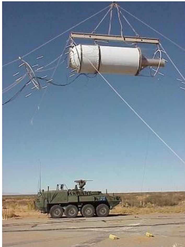
Fig. 8. Test stand for simulating HEMP impact on military machinery
