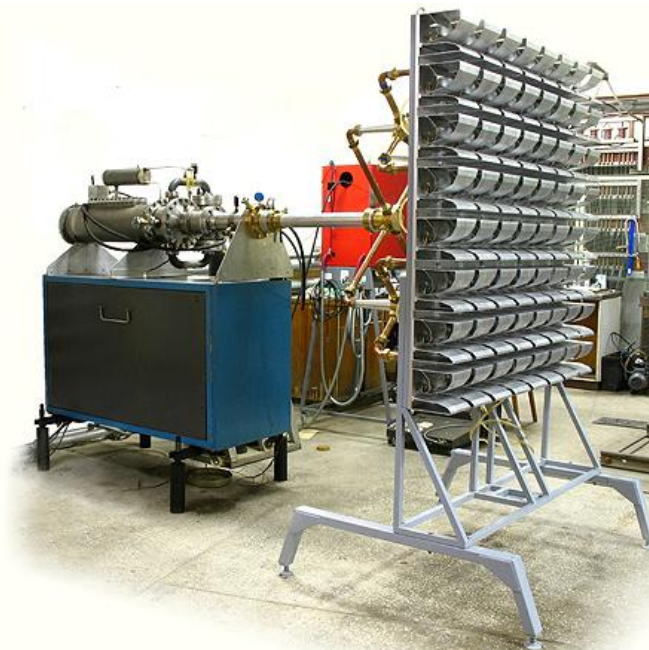
Fig. 5. Generator of ultra wideband pulses with peak radiating power of 3.4 GW developed by Institute of High-Current Electronics of Siberian division of the Russian Academy of Science
