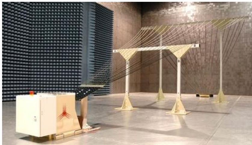
Fig. 11. Test stand available on the market manufactured by Montena Technology (USA) for laboratory testing of large objects, such as relay protection cabinets, for HEMP immunity. On the left – pulse generator, on the right – antenna system.
