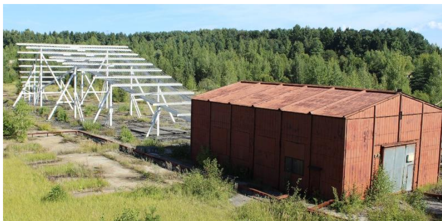
Fig. 9. Stationary HEMP simulator in Test Complex Allur of High-voltage Scientific Research Center of Federal State Unitary Enterprise “All-Russian Electrotechnical Institute” (Istra, Moscow region). Dimensions of simulator: 100 x 35 x 13.5 m, work volume: 10 x 10 x 10 m, pulse shape: 2.5/25 nanoseconds, maximum pulse voltage of electrical field: 70 kV/m.
