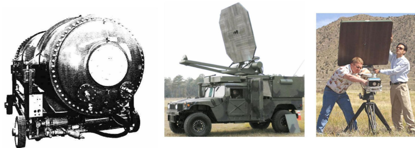
Fig. 6. Left - a super-power mobile high-voltage pulse generator FEBETRON-2020. Output voltage is 2.3 million Volts, the output current is 6000 Amps. In the center - a powerful microwave generator mounted on the car. Right – a transportable powerful microwave generator.
