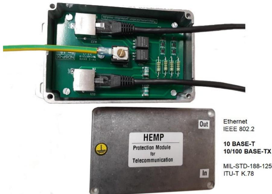
Such a protective module was developed and tested for compliance with standards MIL-STD-188-125 and ITU K.78.
