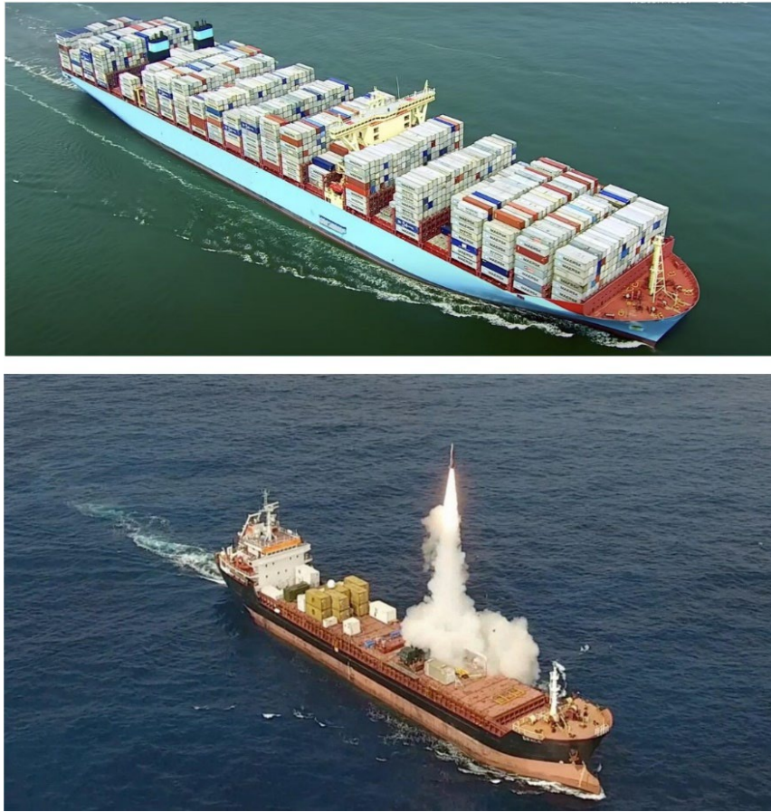
Fig. 4. An ordinary civilian container ship loaded with hundreds of standard containers and a LORA rocket, launched from a ship with containers during a test launch.
