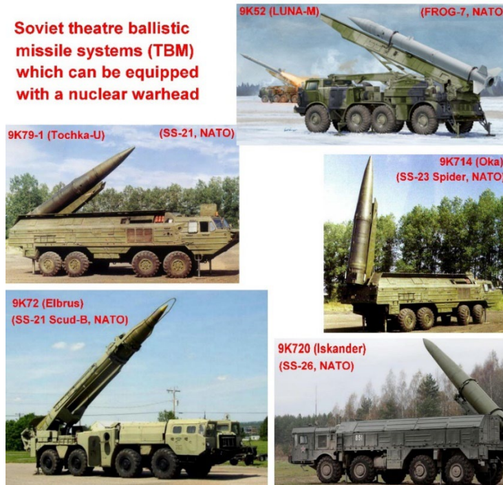
Fig. 3. Soviet/Russian theatre ballistic missile (TBM) systems which can be equipped with a nuclear warhead (explosion yield up to 200 kt).
